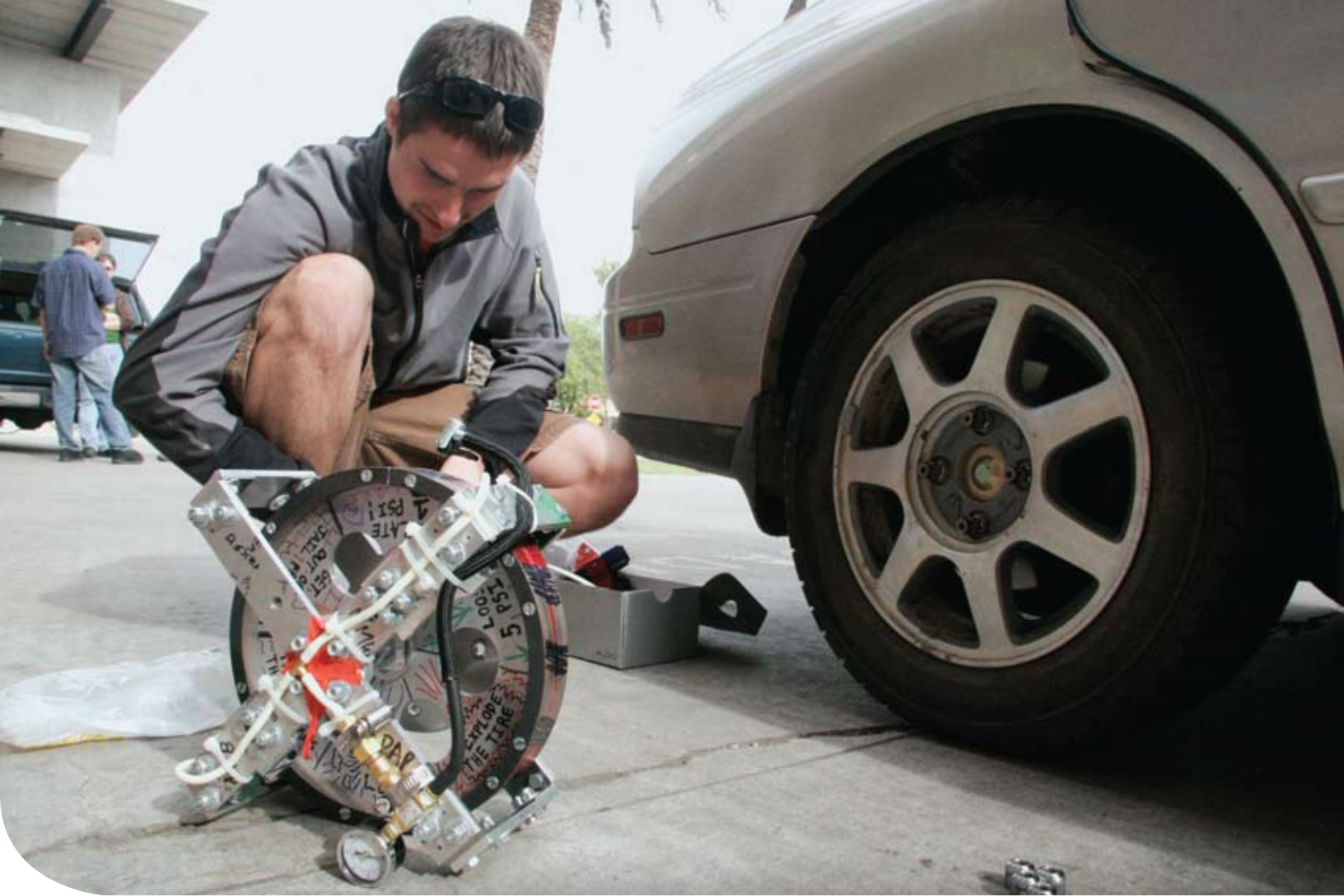
Mechanical engineering student Paul Phelps works on a flywheel-based tire pump device that attaches to an automobile wheel.
